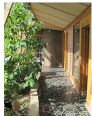
Earthship, Brighton Self-build autonomous house made from recycled tyres and bottles.
